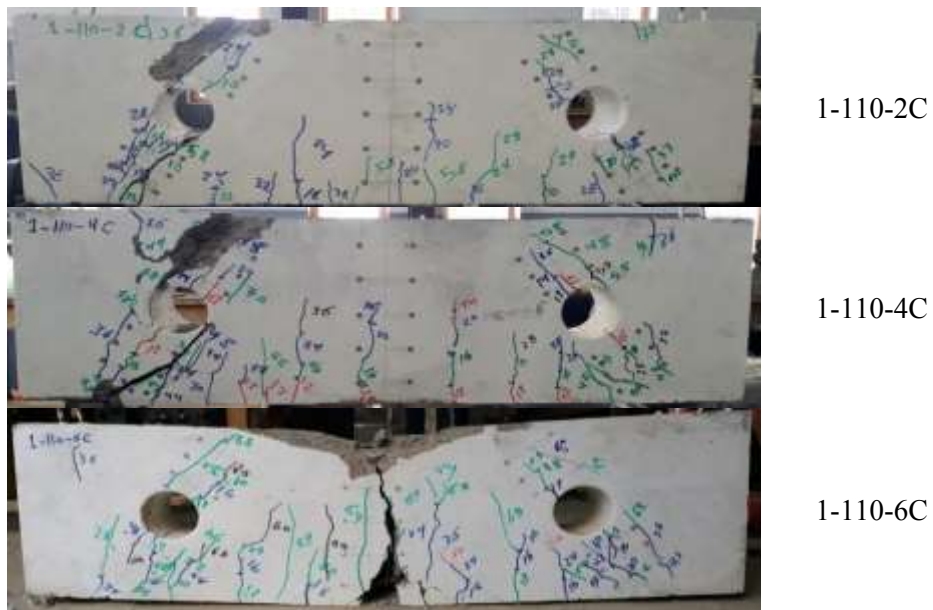
Plate 2-(continued) Deep beams after failure
