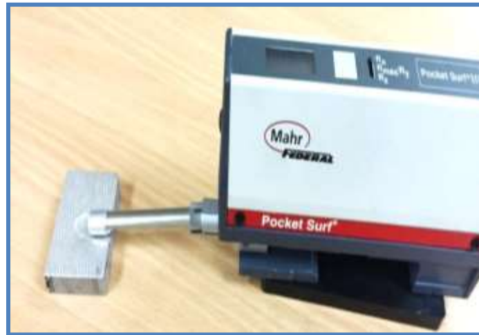
Figure (2): Pocket Surf use in the proposed work for measure surface roughness.
