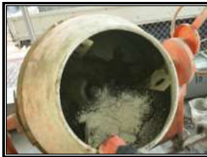
Plate (3): Addition of Foam to the Mix.
