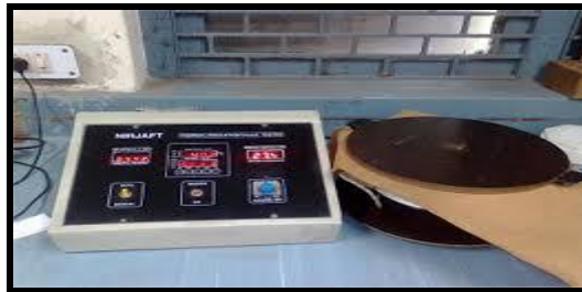
Figure (2) Lee disc thermal conductivity instrument
