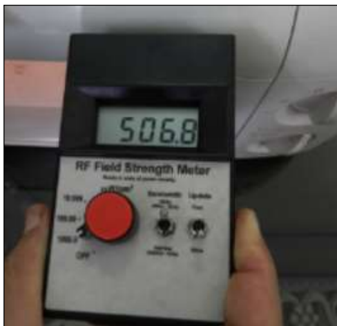
Figure 12: The use of the RF field strength meter to measure leakage from the microwave oven without using the proposed BSF arrays.
