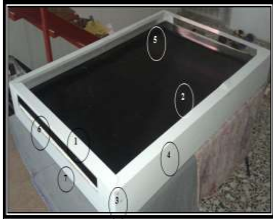
Figure 2: Schematic absorber plate of solar air collector
