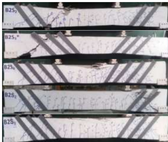
Figure 8: Crack pattern of G3
