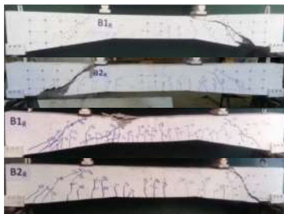
Figure 6: Cracks pattern of group G1
