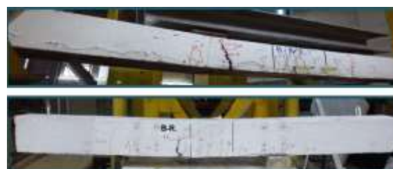
Figure 3: Crack pattern of (B-N.L.) and (B-R.) beams
