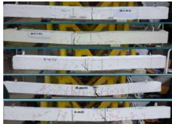
Figure 13: Crack patterns of RPC beams that suffered lap splice failure
