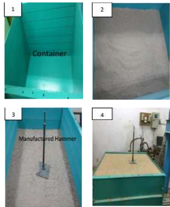
Plate 1: the steps of the sand deposit setup.
