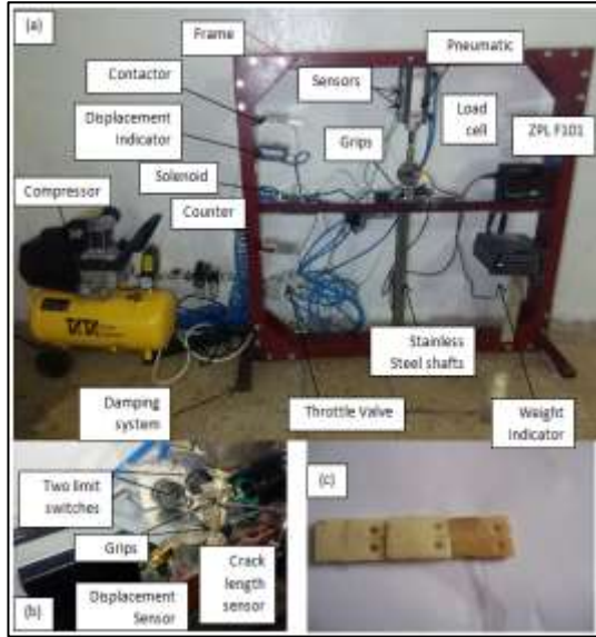
Figure 3: (a) The tensile fatigue rig, (b) the devices about the specimen and (c) The compact tension specimens of human and bovine cortical bone that used in fracture toughness testing
