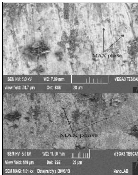
Figure 2: SEM for Sample Ti_2AlC cold pressed and sintered at 1400°C for 4hr
