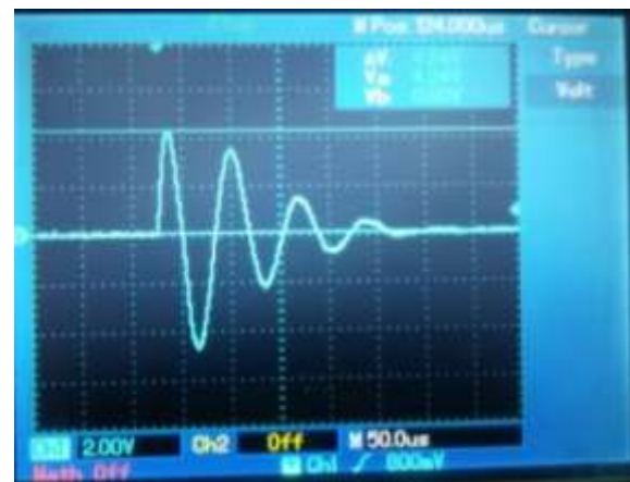
Figure 1: Current waveform of copper wire explosion (Peak voltage)
