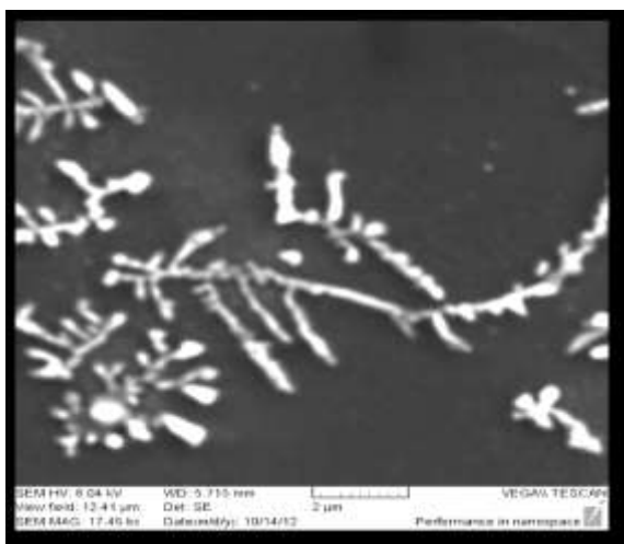
Figure 3: SEM micrographs of the prepared AgNPs using first method (AgNPs) at T=100^{\circ}\text{C}
