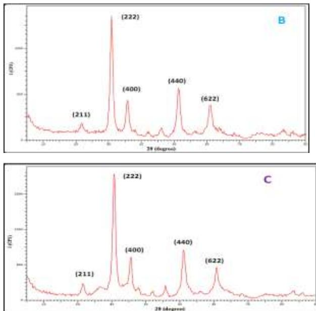
**Figure 2: XRD patterns of the particles (a):ITO 20% (b): ITO 40% mole at 400 °C**
