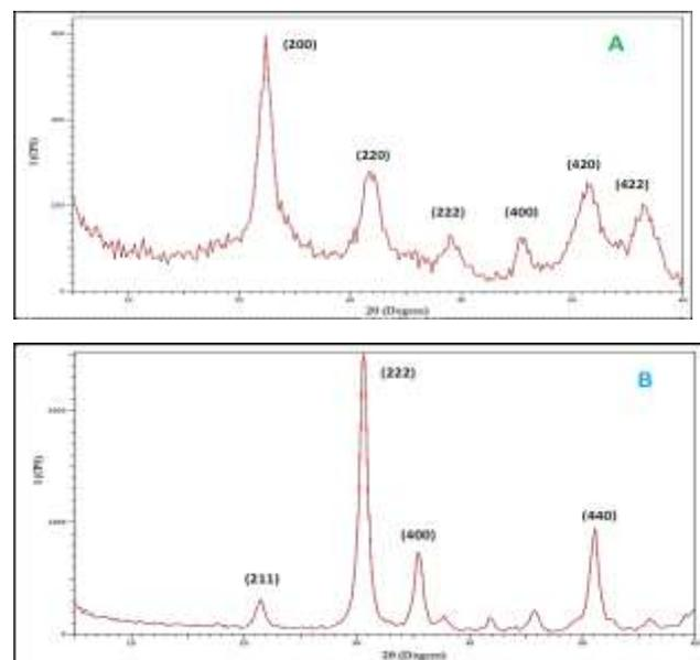
**Figure 1: XRD patterns of the particles (a):  $\text{In}(\text{OH})_3$  at 200 °C (b):  $\text{In}_2\text{O}_3$  at 400 °C**
