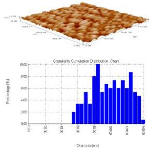
**Figure 3: AFM images 3D and B- granularity cumulation distribution chart of In<sub>2</sub>O<sub>3</sub> annealed at 400 °C.**
