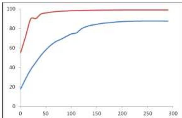
**Figure 6: Sensitivity of  $\text{In}_2\text{O}_3$  and ITO thin films annealed at  $400^\circ\text{C}$  for CO gas. (where X-axis is sensitivity and Y-axis is time(sec)).**
