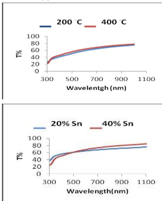
Figure 5: UV-VIS transmittance spectra of In<sub>2</sub>O<sub>3</sub> thin films: (a) at different annealing temperature (200 and 400 °C), (b) at different compositions (20 and 40% mole) with Tin Oxide.
