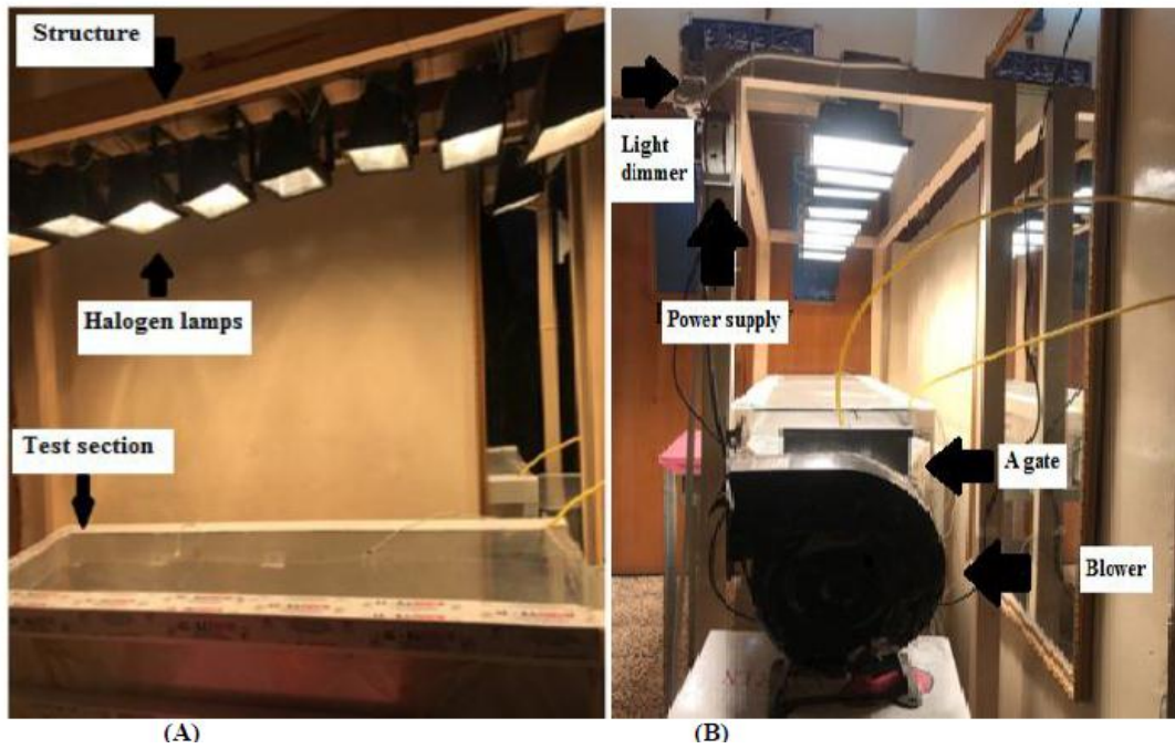
Figure 1: Experimental Setup (A) the front side and (B) the view side
