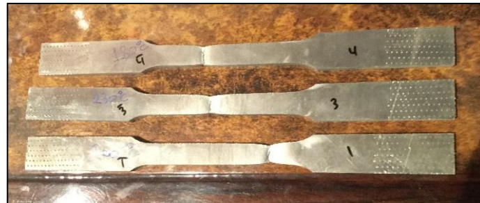
Figure 9: Specimens were tested at different temperatures.
