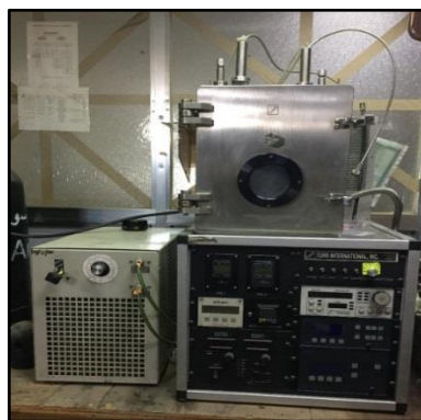
Figure 1: RF Magnetron sputtering system.
