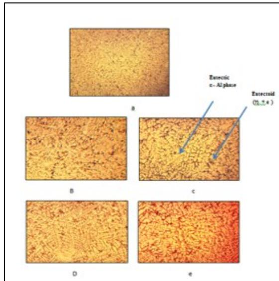
**Figure 7: Microstructure of ZA-27 alloy- matrix with nano particles at different weight percent**
