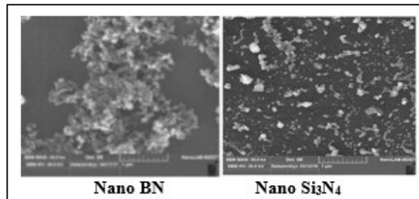
Figure 1: SEM of nano BN and  $\text{Si}_3\text{N}_4$  nano powders
