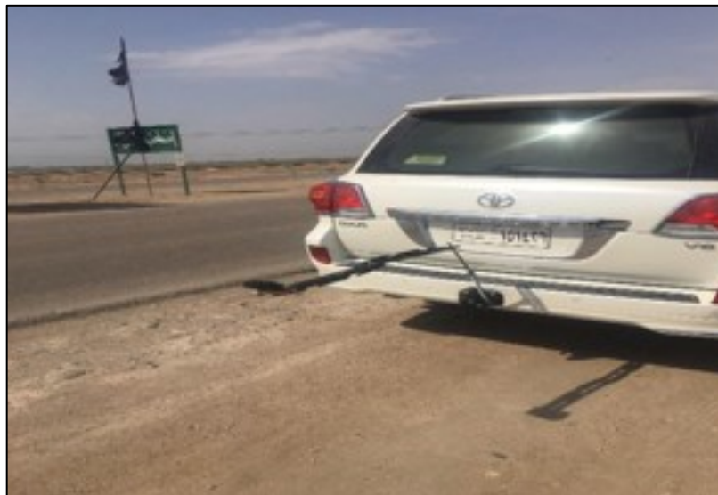
Figure 8: The stand of camera on the vehicle
