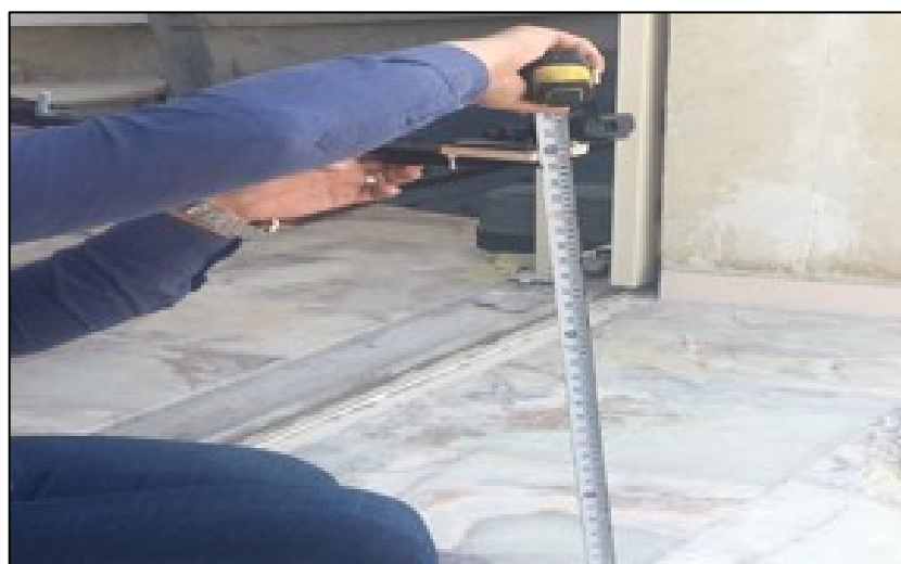
Figure 9: The height of camera from the face of pavement (96cm)
