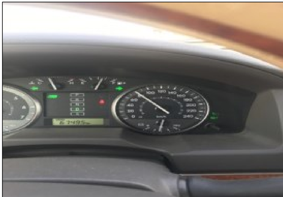
Figure 11: The cruise control of vehicle speed on 80kmph
