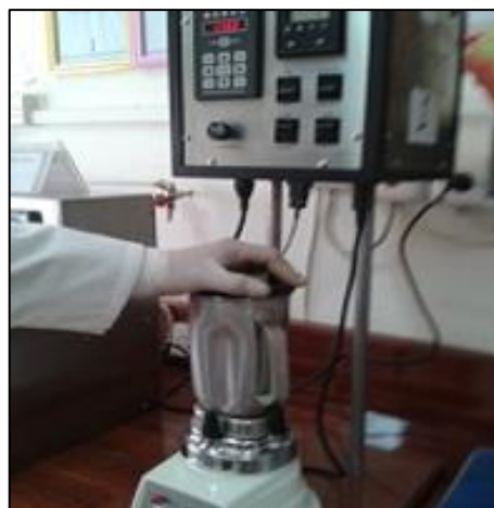
Fig. 3: Mixing cement slurry
