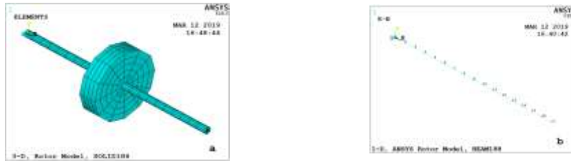
Figure 4: ANSYS rotor model, a: 3-D, model using solid186, b: 1-D, model using beam188
