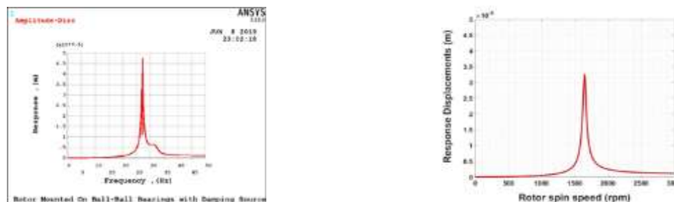
Figure 11: Response of rotor Mounted on ball bearings with an external damping source
