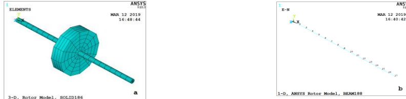
Figure 4: ANSYS rotor model, a: 3-D, model using solid186, b: 1-D, model using beam188
