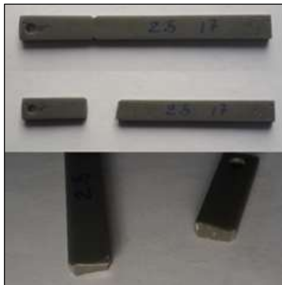
Figure 5: Notched fatigue specimen before and after being tested
