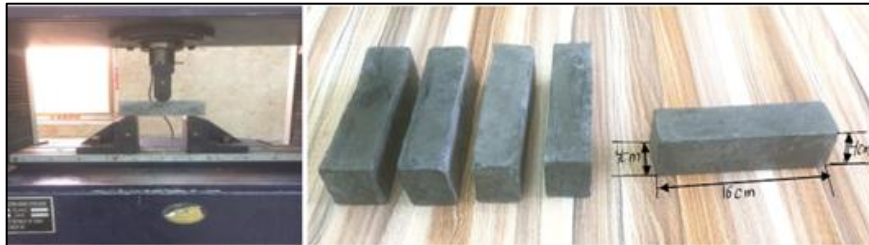
Figure 8: shows the samples of CNTs/SiO 2 substituted cement mortar in the bending test
