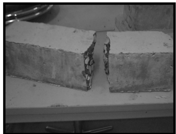
Figure 12: Shows a A4 beam after flexural strength test
