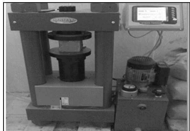
Figure 8: A cube during the compressive strength test
