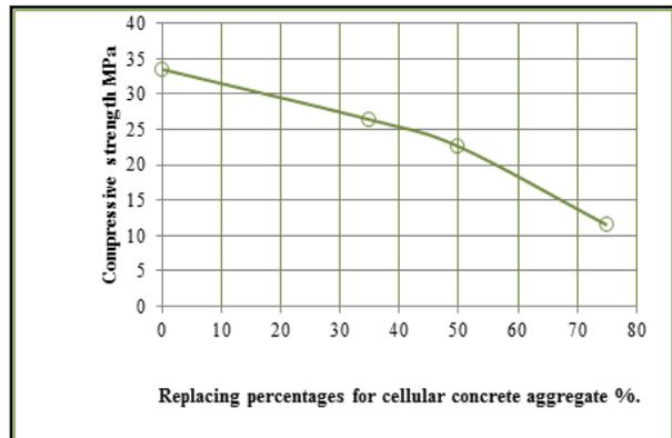
Figure 6: Relationship between compressive strength and replacing percentages for cellular concrete aggregate
