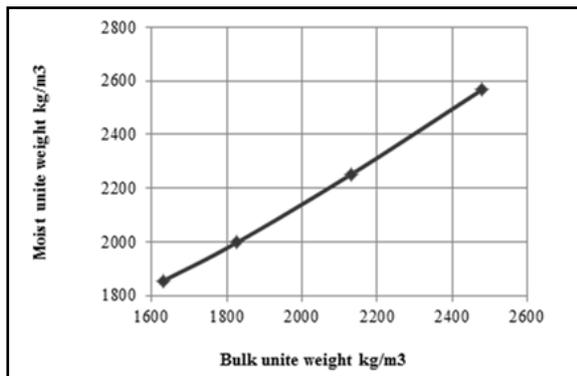
Figure 5: Relationship between bulk density and moist density for all mixes
