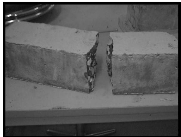
Figure 12: Shows a A4 beam after flexural strength test
