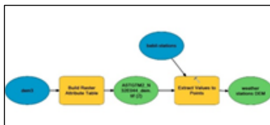
Figure 6: model to extract Digital Elevation Model for the weather station
