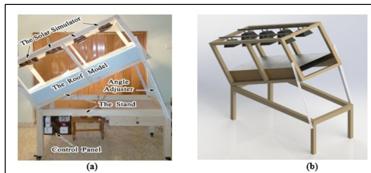
Figure 2: The experimental rig. (a) Photographic image. (b) Isometric view
