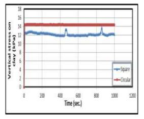
Figurer 13: Vertical Stress Change with Time when cu = 20 kPa,  $D_f = 0$  cm, Velocity = 6 mm/sec at Depth 10 cm
