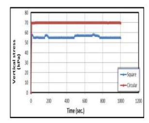
Figure 20: Vertical Stress Change with Time when cu = 70 kPa,  $D_f = 0$  cm, Velocity = 6 mm/sec at Depth 10 cm
