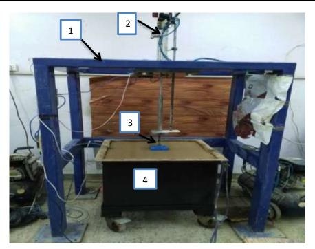
Figurer 1: Overall outlook of the produced device: 1. Steel load framing, 2. Axial load system, 3. Model footings, 4. Steeling box (test container)
