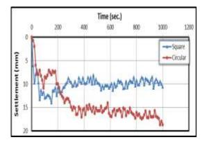
Figurer 12: Settlement Change with Time when the  $D_f = 5$  cm, cu = 70 kPa and Velocity = 6 mm/sec.
