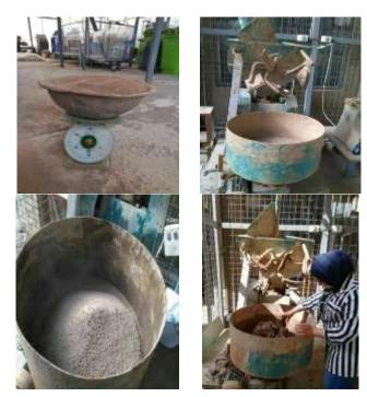
Figurer 2: Preparation of Clayey Soil by Grinding
