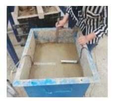
Figurer 5: Installing Pressure Cells and Piezometer and Checking the Distance from the Surface to the Sensors Equal to 2B= 20 cm
