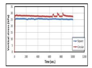
Figure 18: Vertical Stress Change with Time when cu = 40 kPa,  $D_f = 5$  cm, Velocity = 6 mm/sec at Depth 10 cm
