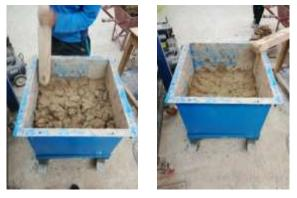
Figurer 3: Placing the Clay in the Box and Compaction Gently by Wooden Tamper to Avoid the Entrapped Air
