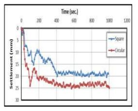
Figurer 9: Settlement Change with Time when the  $D_f = 0$ , cu = 70 kPa and Velocity = 6 mm/sec.
