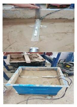
Figurer 6: Installing Pressure Cells and Piezometer and Checking the Distance from Surface to Sensors Equal to B= 10 cm
