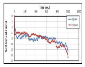
Figurer 10: Settlement Change with Time when the  $D_f = 0$ , cu = 40 kPa and Velocity = 6 mm/sec.
