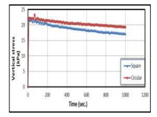
Figure 19: Vertical Stress Change with Time when cu = 40 kPa,  $D_f = 5$  cm, Velocity = 6 mm/sec at Depth 20 cm
