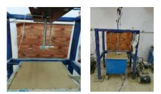
Figurer 4: Surface Adjustment of the Model and Carrying the Model into the Load Setup.
