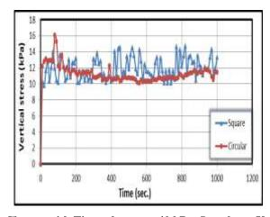
Figure 17: Vertical Stress Change with Time when cu = 40 kPa,  $D_f = 0$  cm, Velocity = 6 mm/sec at Depth 20 cm
