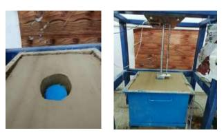
Figurer 7: Footing at Surface and at Depth 5 cm
