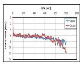
Figurer 11: Settlement Change with Time when the  $D_f = 5$  cm, cu = 40 kPa and Velocity = 6 mm/sec.
