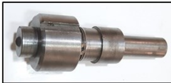
Figure 4: Tool burnishing used in the experimental study
