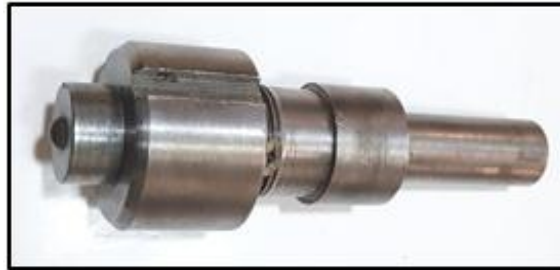
Figure 4: Tool burnishing used in the experimental study
