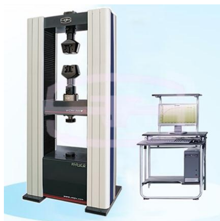
Figure 2: Universal testing machine WDW model (200E) electromechanical load frame with mechanical grips
