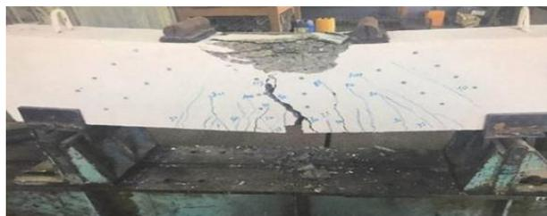
**Plate 6: Cracks pattern of beam B5**
