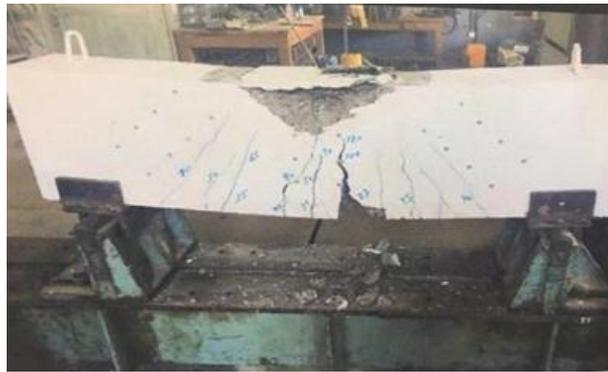
Plate 7: Cracks pattern of beam B6
