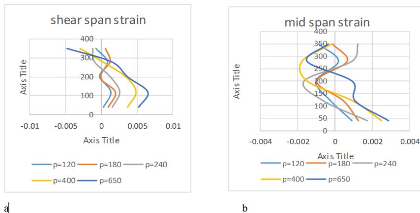
Figure 5: Concrete surface strain of beam a. C-B1 at mid span, b. C-B1 at shear span
