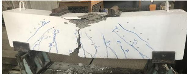
**Plate 3: Cracks pattern of beam B2**
