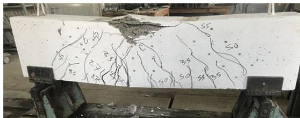
**Plate 4: Cracks pattern of beam B3**
