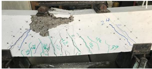
**Plate 2: Cracks pattern of beam C-B1**
