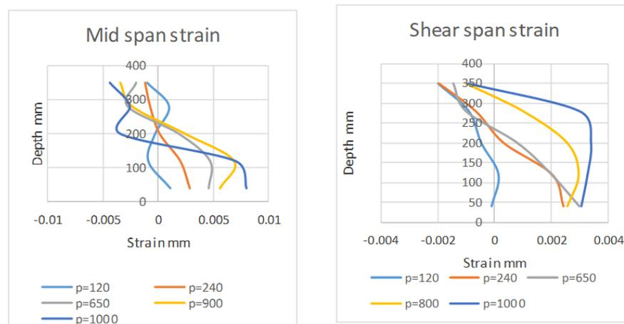
**Figure 6: concrete-surface-strain beam with strut reinforcement confinement (B2)**
