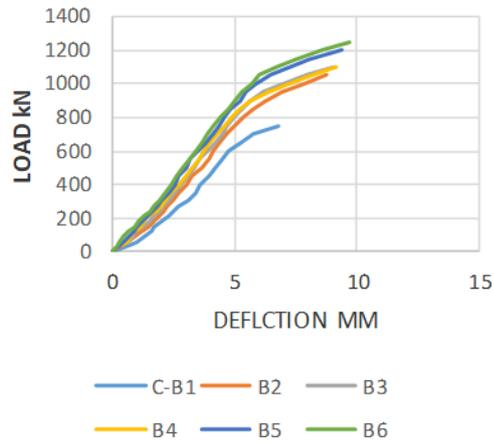
Figure 4: (Load-deflection)-curves of deep beams specimens
