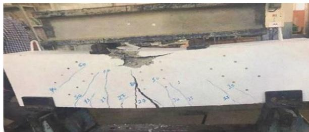
**Plate 5: Cracks pattern of beam B4**
