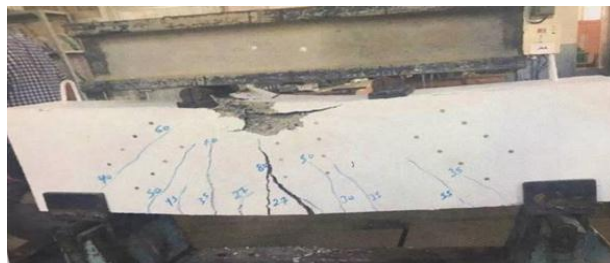
Plate 5: Cracks pattern of beam B4
