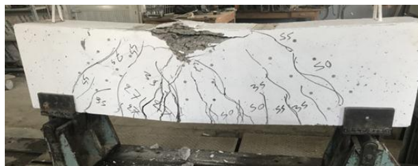
Plate 4: Cracks pattern of beam B3
