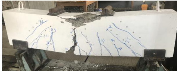
Plate 3: Cracks pattern of beam B2
