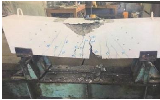
Plate 7: Cracks pattern of beam B6
