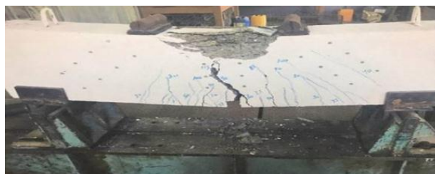
Plate 6: Cracks pattern of beam B5
