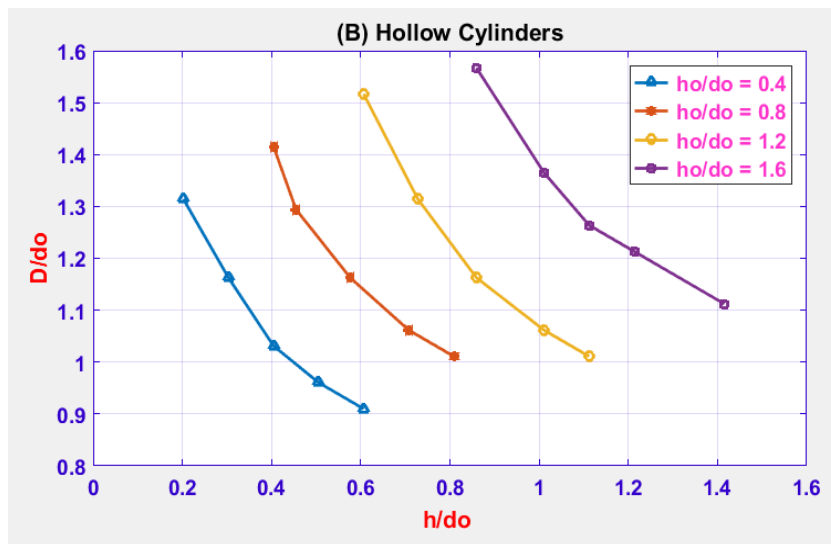
Figure 4: Experimental Variation of Diameter Ratio (D/do) with Respect to Non-Dimensional Height (h/do) for Different Aspect Ratios (ho/do) {A-for Solid Cylinder and B-for Hollow Cylinder}
