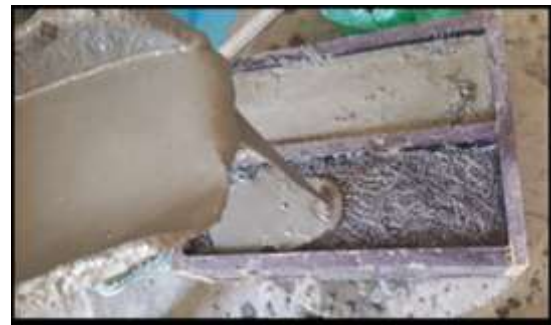
Figure 5: the casting procedures of SIFCON
