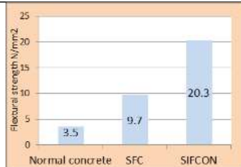
Figure 8: Flexural strength at 28 days age
