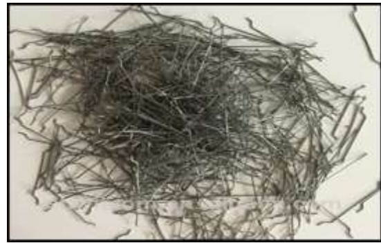
Figure 4: Steel fiber used in this research
