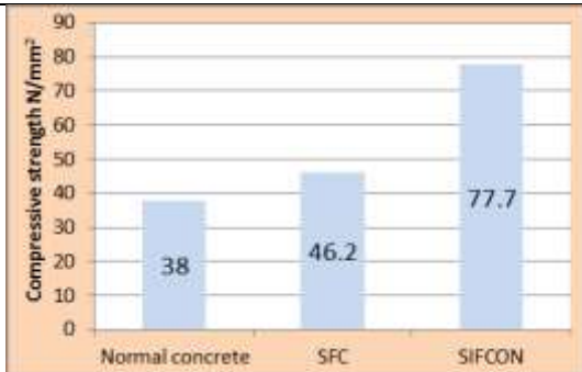
Figure 7: compressive strength at 28 days age
