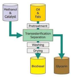
Figure 3: The schematic of biodiesel preparation
