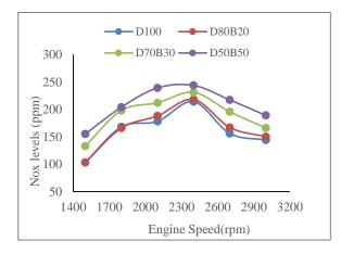
Figure 9: The engine speed impact on the (NO<sub>x</sub>) levels emitted for studied blends
