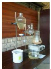
Figure 2: The biodiesel preparation system
