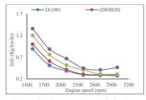
Figure 4. The impact of engine speed on the (BSFC) of tested blends
