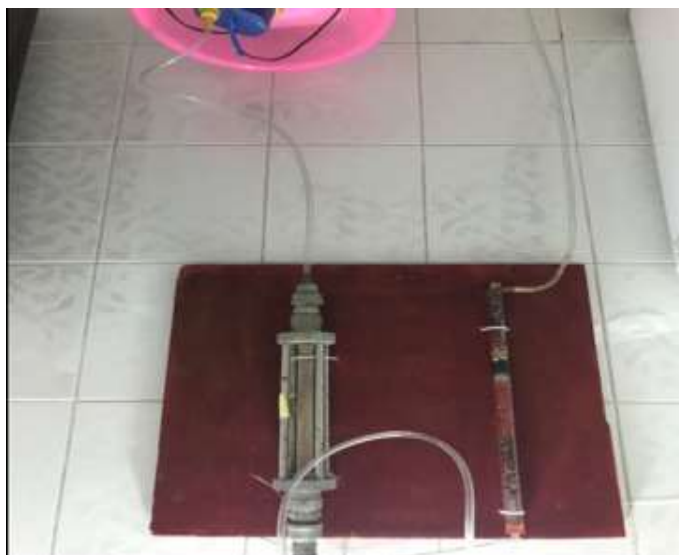
Figure 3: show the packed bed reactor
