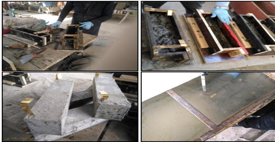
Figure 3: Preparation of smart cementitious composites sensors
