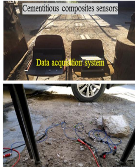
Figure 7: Measurement of axle load in motion by self-sensing specimens
