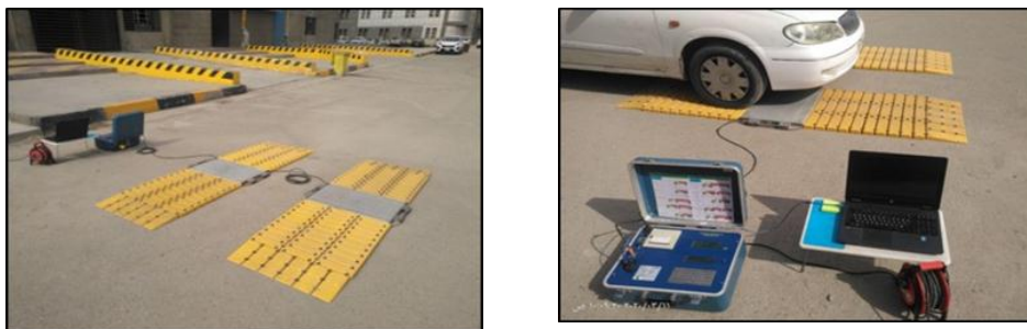
Figure 4: Measurement of axle load in motion by WIM system
