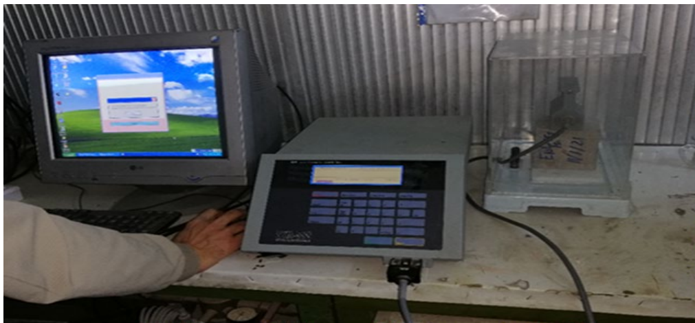
Figure 5: Thermal conductivity test of concrete specimen
