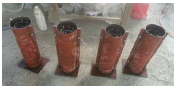
Figure 2: Assembled column moulds
