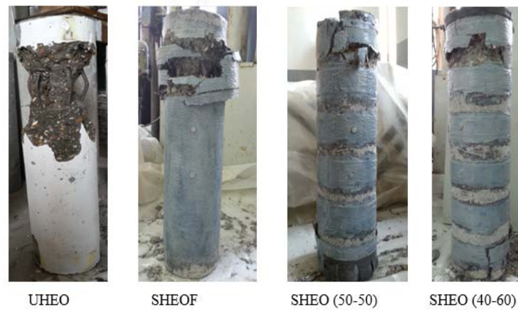
Figure 7: Failure pattern for HPCEO columns
