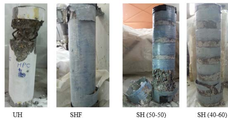
Figure 8: Failure pattern for HPC column
