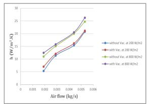
Figure 11: Variation for coefficient of heat transfer (W/m<sup>2</sup> K) with air flow of the solar collector at different values of irradiance
