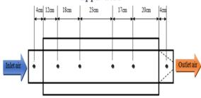
Figure 3: Thermal sensor distribution network on design
