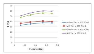
Figure 7: Variation of the temperature of glass cover with distance of the solar air collector at different irradiance values with and without vacuum
