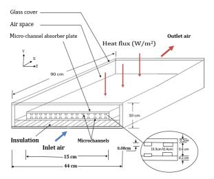
Figure 4: Sketch of solar collector with microchannels absorber plate
