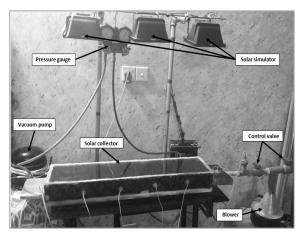
Figure 1: Photograph of the experimental apparatus
