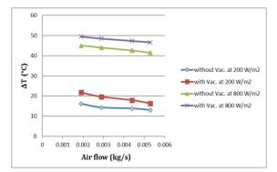
Figure 9: Experimental variance of temperature difference of air  $\Delta T$  (°C) with air flow at different values of irradiance with and without vacuum
