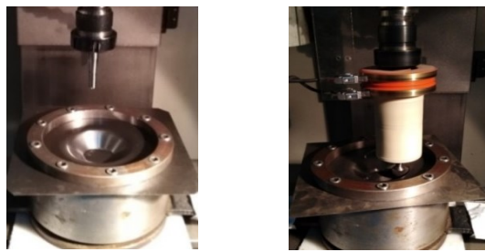
Figure 2: A: SPIF tool and B: MAF tool
