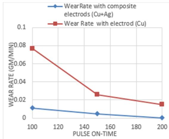
Figure 8: Effect Plus (Time - On) on TWR
