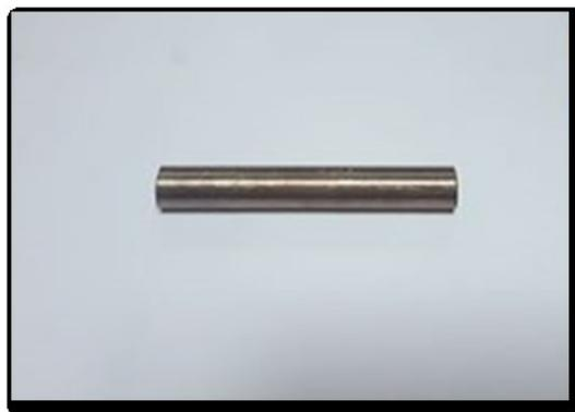
Figure 1: Composite Electrode Copper: Silver (70:30)
