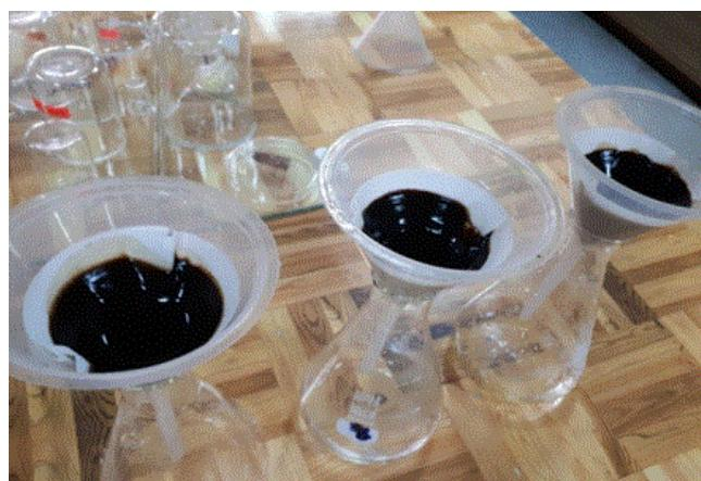
Figure 3: Iron particles separated by filter paper of  $0.45\mu\text{m}$  pore size
