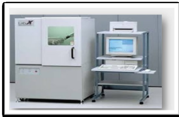
Figure 4: X-ray diffraction device of residual stresses measuring
