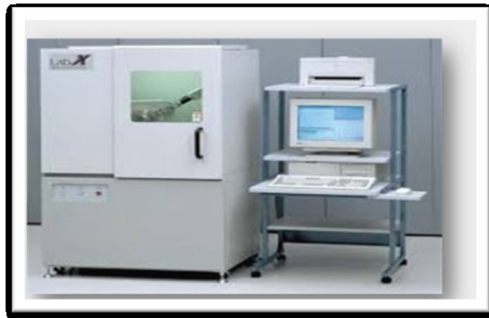
Figure 4: X-ray diffraction device of residual stresses measuring
