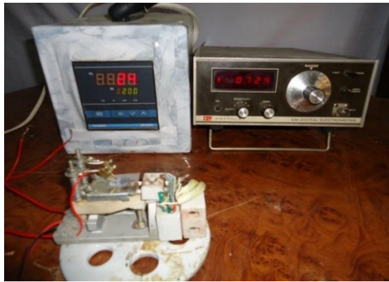
Figure 8: Photograph represents a home-made thermal and electrical measurement stage.
