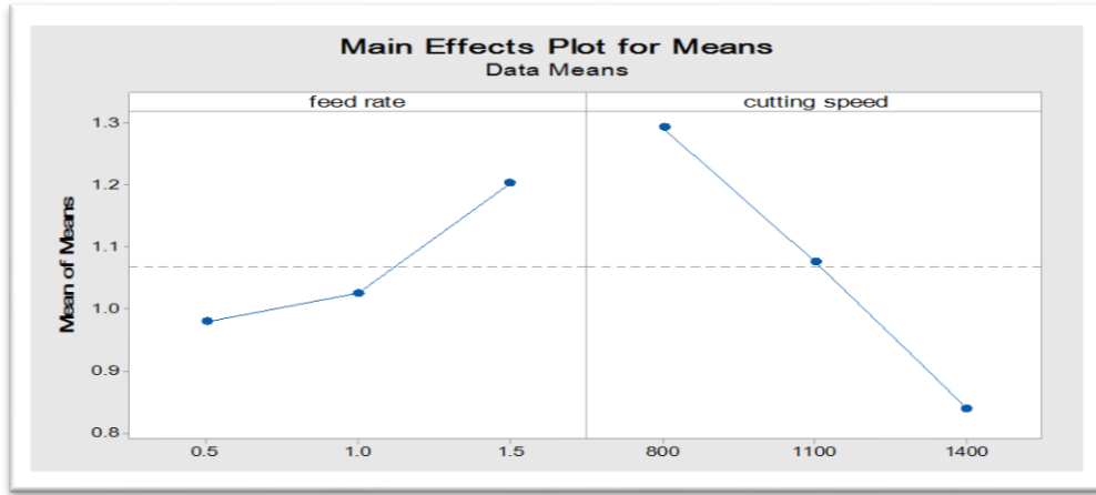
Figure 6: Effect of the cutting speed & the feed rate on SR using Al 2 O 3 coated cutting tool.
