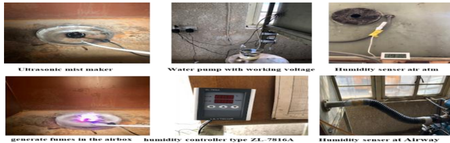
Figure 7: Steps of installing the ultrasonic mist maker device in the intake airbox.
